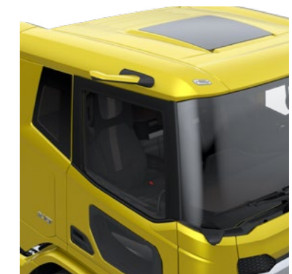
CAMERAS & CORNER VIEW
