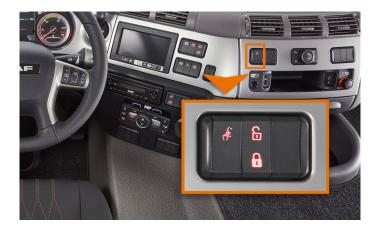
The second part is the silent function in the engine software that is activated by the silent switch on the dashboard. If activated the engine software limits the maximum engine speed and engine torque, which results in a lower noise level. The DAF silent solution fits within DAF's responsibility to build vehicles that are environmental friendly and sustainable.
